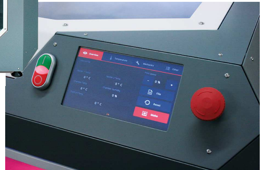
HMI of the developed control system
